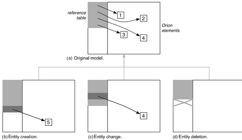
Fig. 3. Illustration of Orion dynamics through different changes (creation, change, deletion).
