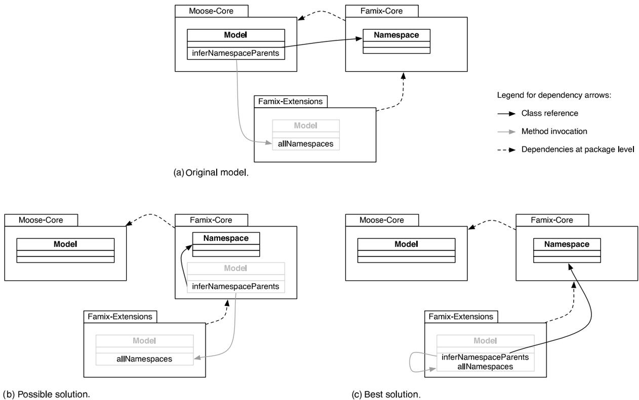
**Fig. 1.** (a) Two circuits between three packages; (b) a change that removes two circuits but creates a new one; (c) a change that effectively removes two circuits.
